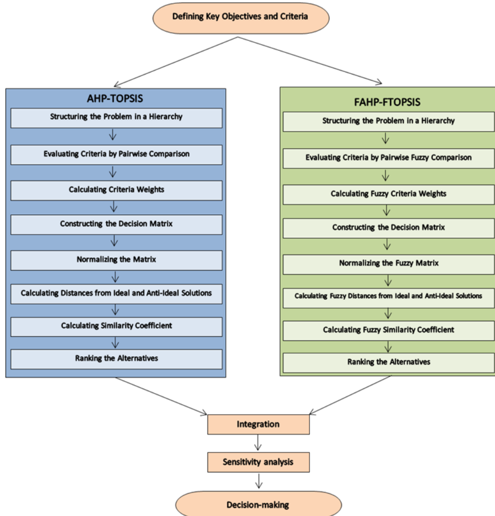
Figure 1. Integrated Workflow of AHP-TOPSIS and FAHP-FTOPSIS
